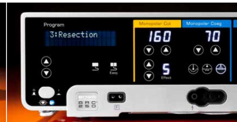
The resection program provides a default setting for the use of monopolar resectoscopes or hysteroscopes of up to max. 250 W
